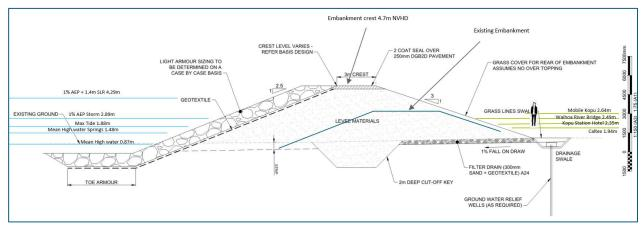
Figure 41: Possible future coastal defence crest level for Kopu compared to oceanic and landside elevations
