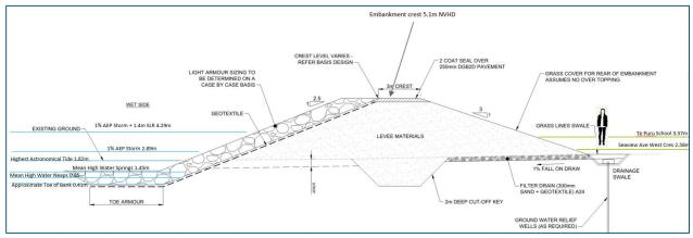
Figure 22 Te Puru possible defence crest levels compared to oceanic and landside elevations
