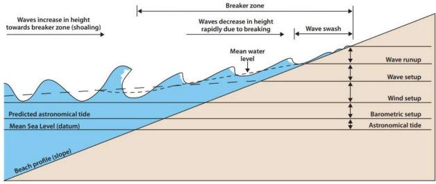
Figure 3: Storm tide schematic
