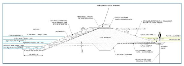
Figure 36: Thames possible coastal defence crest levels compared to oceanic and landside elevations
