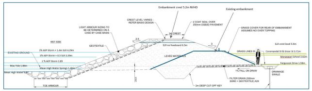
Figure 32 Moanataiari possible defence crest levels compared to oceanic and landside elevations
