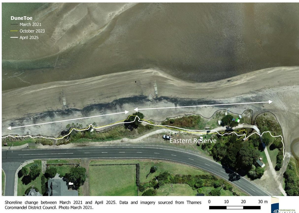
Figure 9: Change in dune toe position over monitoring period. Note severe erosion adjacent to and east of the eastern groyne.
