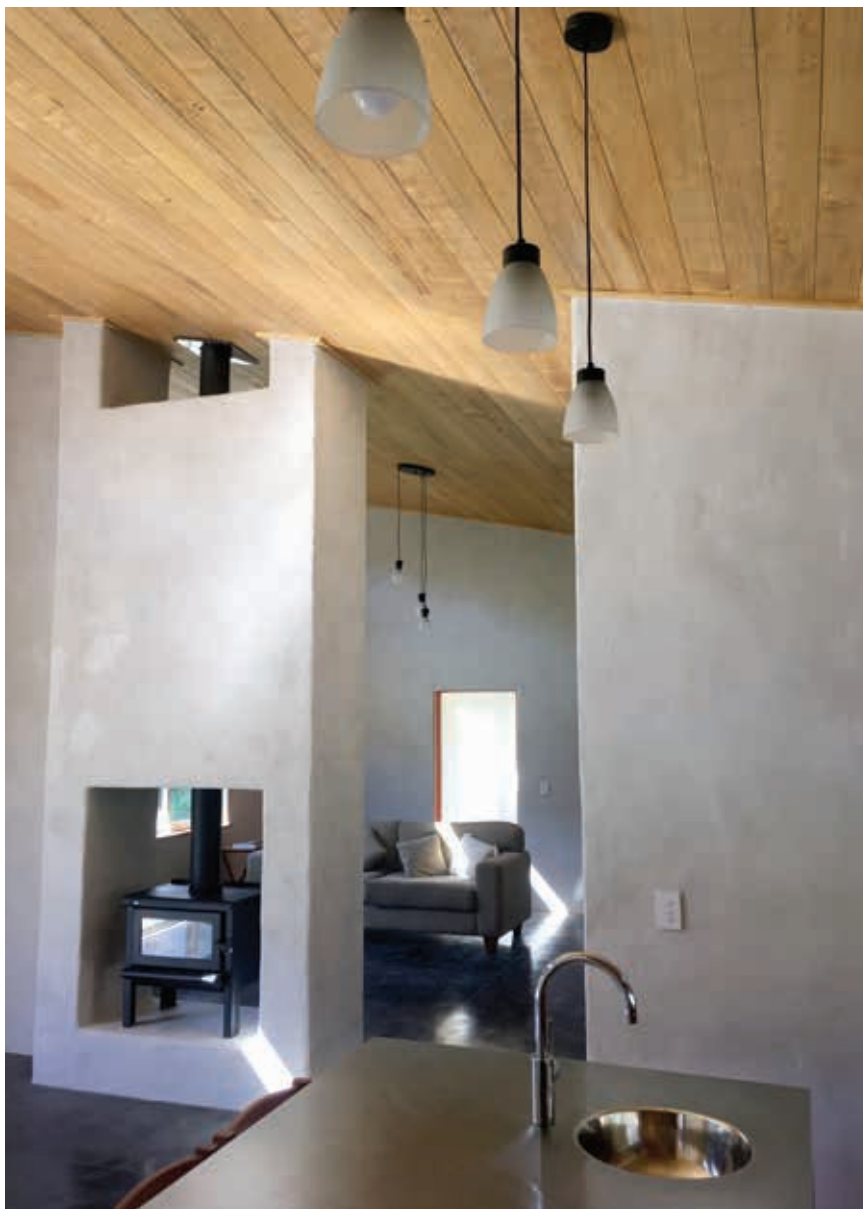
▼ Stained concrete floors absorb heat and release it at night. A wood stove provides backup heating.
