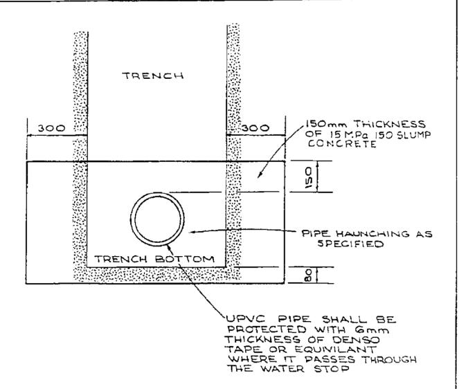
I. WATER STOPS SHALL BE CONSTRUCTED IN THE TRENCH WHERE SHOWN ON THE PLAN OR WHERE ORDERED BY THE ENGINEER.
