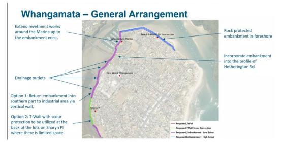
General arrangement plan - protection for larger extent than the inundation extent than
